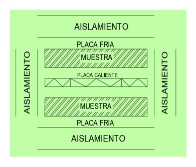
The design has a thermal protection on the side of the prototype, insulated with refractory ceramic fiber, this insulation is placed on the 4 sides of the prototype including both the base where the lower cold plate and the upper cold plate are placed.
